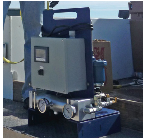
Figure 2 | An innovative membrane technology designed to assist in moisture control. (Courtesy of Compact Membrane Systems, Inc.)
